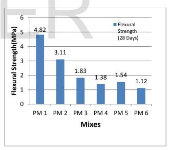
The flexural strength graph shows a depreciation of strength throughout. For PM 1 mix it showed the highest of 4.82 MPa. For PM 2, 55% reduction in strength was observed. For PM3 and PM 4 mixes containing FA compared to PM 1 showed gain in strength only about 38% and 28.6%. For mixes PM 5 and PM 6 containing GGBS also showed lower strength. Gain in strength was only 32% and 23.2% respectively with respect to PM 1.
