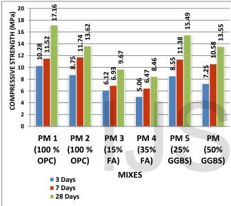
The pervious concrete showed significantly lower strength. The mean value of the 28 days compressive strength of pervious concrete with 100% cement had 17.16 MPa for 10mm aggregate and 13.62 MPa for mix of 10 and 20mm aggregate. As expected, pervious concrete resulted in 26% low compressive strength due to its higher porosity. Further, the samples were prepared using 10 mm aggregates.
