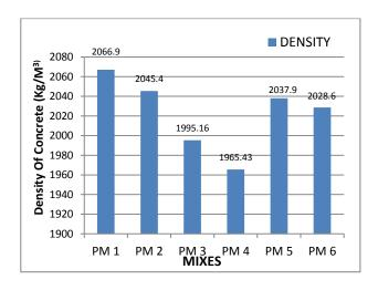
The mean density for conventional concrete varies between 2400 and 2500 kg/m³, while pervious concrete has a density between **1965 and 2067 kg/m³**. Therefore, the pervious concrete showed nearly **21-27%** lower density than conventional concrete. The age of concrete does not influenced to the density of pervious concrete. The cement replacement with fly ash and GGBS had marginally affected decreasing the density for both pervious concretes.
